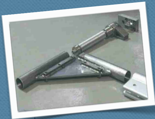
Return spring system & Junction tubes
